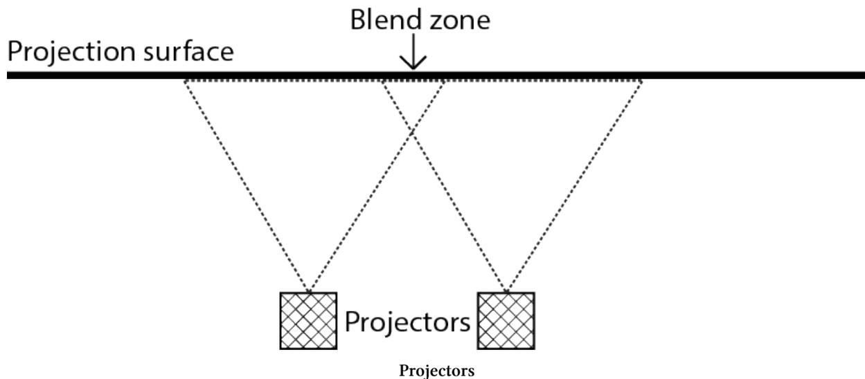
If the amount of pixels in the blend zone are already known, input them into the 'Region' parameter of the 'EdgeBlend' component. Then try turning off the 'Enable Blend' button to make sure your image is correctly overlapping. At this point, the overlapped images should match and be lined up. Always remember the main purpose of an edge blending tool is to remove the seams, not line up the content.
