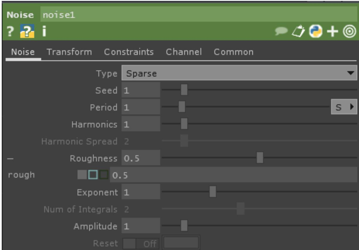
There are three main elements that are available once a parameter is expanded. The first on the left, is the parameter's scripting name. This scripting name is needed whenever that parameter is referenced in any of TouchDesigner's scripting languages. In the above diagram, the scripting name for the Noise CHOP's Roughness is 'rough'. Continuing the above example, the Python script to set the Roughness of the above Noise CHOP to '1' would be:
