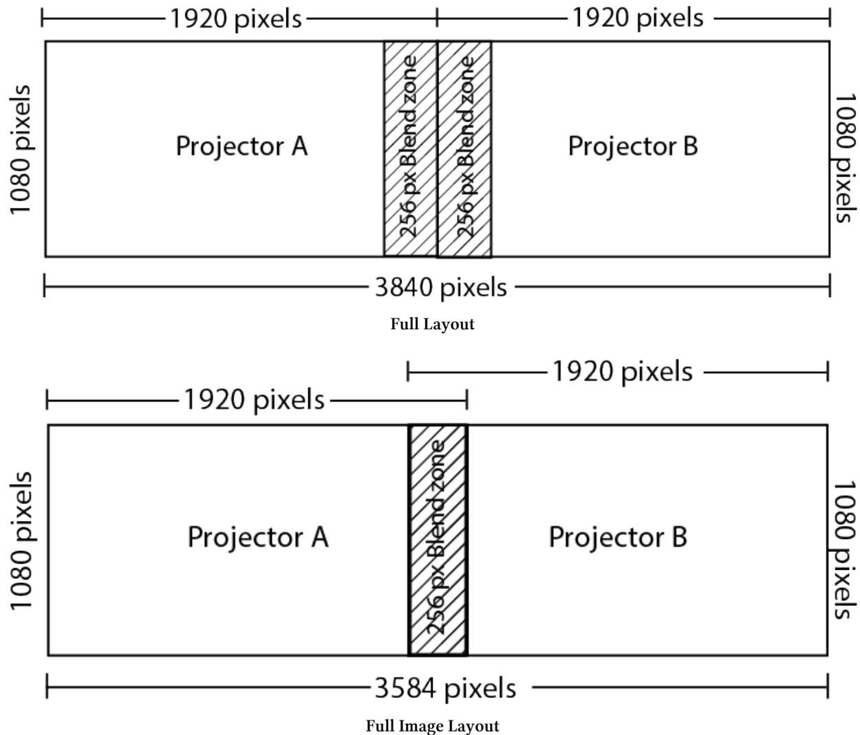
Implementing this example is straightforward in TouchDesigner thanks to built-in edge blending tools. Before using the built-in edge blending component, let's take a look at the base elements of an edge blending workflow in a simple example.
