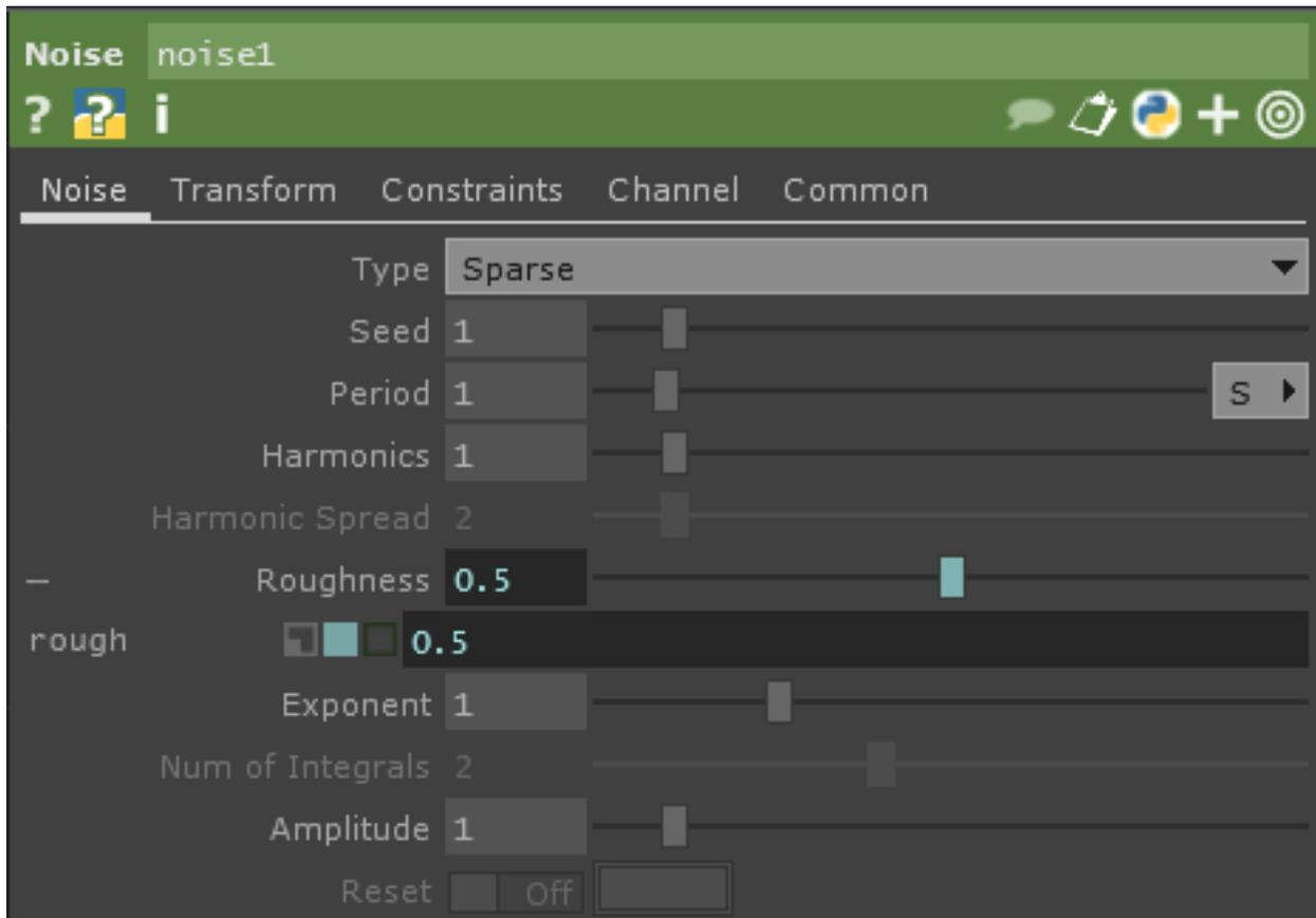
To change the parameter's mode to Export mode, a CHOP channel needs to be dragged and dropped on the parameter, at which point it will take up Export mode's colour scheme, and the green box will be filled in.
